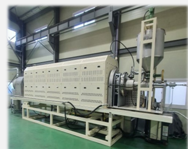
<Rotary Kiln Type Activation Furnace>
