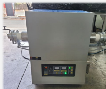
<Tube Type Furnace (~1,400°C)>
