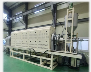
<Rotary Kiln Type Activation Furnace>
