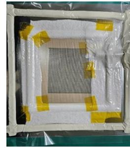
Figure 2. Sample with vacuum before curing in oven
