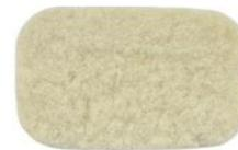
Fig. 2. Freeze-dried Porous pulp.
