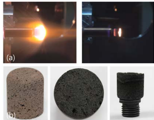
Fig. 1. (a) Arc-jet test and (b) Specimen B/A
