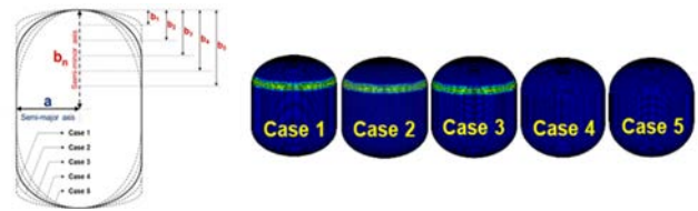
Fig. 2. 1 st Buckling Mode by Elliptical Ratio.
