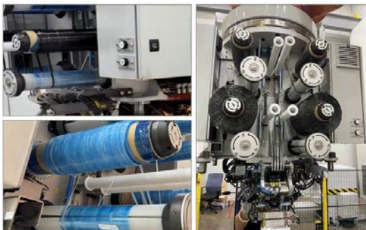
Fig. 1. AFP Equipment with Prepreg and Towpreg Installed.
