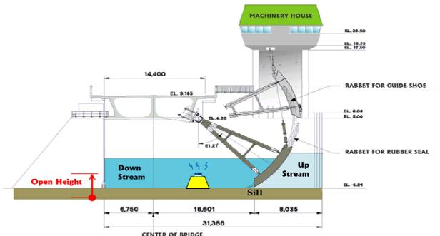
Fig. 4. Flow rate measuring equipment installation sectional view.
