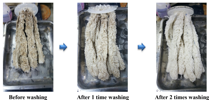
Fig. 11. Filter cleaning using hand washing method
